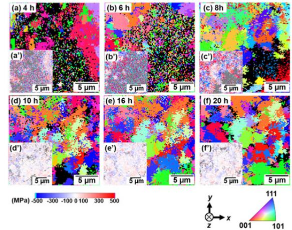
Fig. 2. (a)–(f) Crystallographic orientation maps of electroplated Cu at  $t =$  (a) 4 h, (b) 6 h, (c) 8 h, (d) 10 h, (e) 16 h, (f) 20 h. (a')–(f') Deviatoric stress maps ( $\sigma_{zz}$ ) corresponding to (a)–(f), respectively. The dark/gray pixels were the unresolved area.
