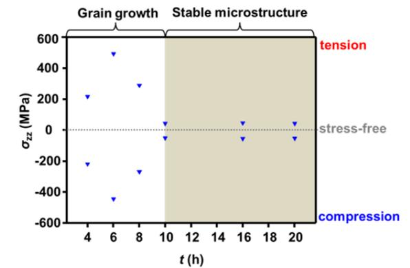
Fig. 3. Deviatoric stress ( $\sigma_{zz}$ ) of electroplated Cu as a function of  $t$ .
