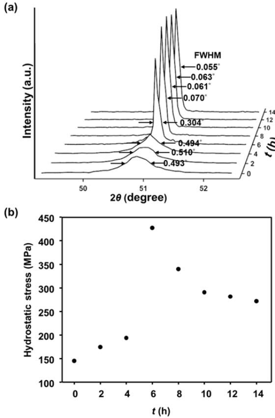
Fig. 1. (a) In-situ synchrotron X-ray diffraction spectra of electroplating Cu upon self-annealing.; (b) Hydrostatic stress of electroplated Cu as a function of  $t$ .
