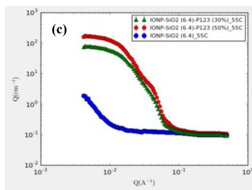
Fig. 2. SANS spectra of IONP-SiO<sub>2</sub>, IONP-SiO<sub>2</sub>-P123 (30%) and (50%) at 55°C.
