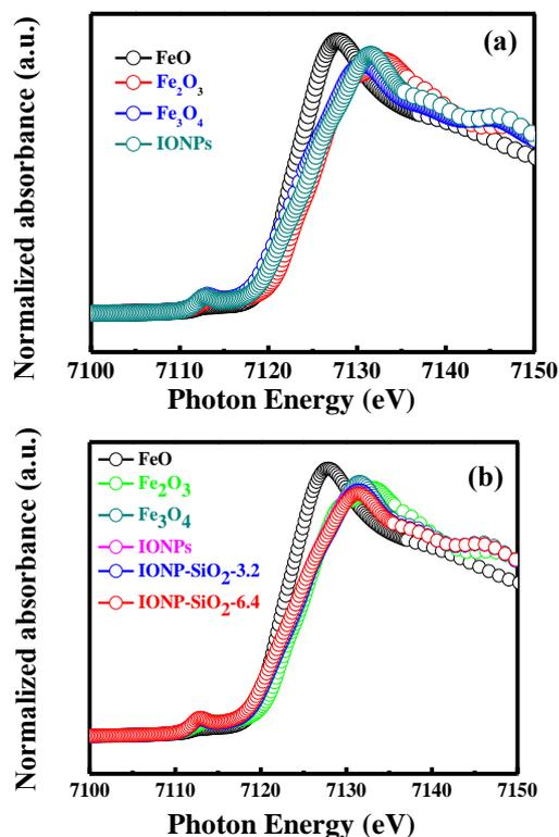
Fig. 1. (a) Fe K-edge XANES spectra of IONPs compared to different iron standards and (b) XANES spectra Fe, FeO, Fe<sub>2</sub>O<sub>3</sub>, Fe<sub>3</sub>O<sub>4</sub> and IONP-SiO<sub>2</sub> at different concentrations of SiO<sub>2</sub>.
