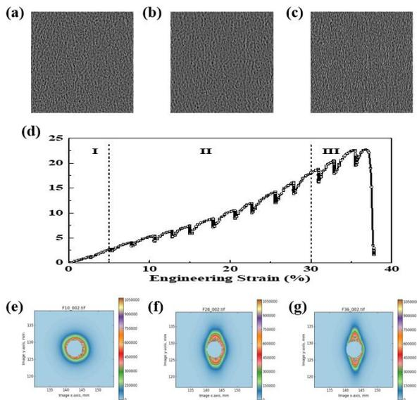
Fig. 2. (d-f) (a-c) TXM images of underneath annealed P(VDF-TrFE) nanofibers orientation during the three regions of uniaxial tensile test. (d) The engineering stress-strain (S-S) curve. (e-g) The 2D SAXS patterns.
