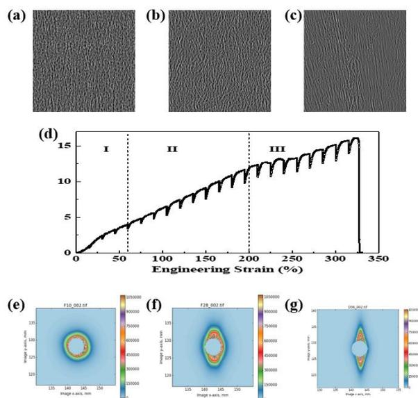
Fig. 1. (a-c) TXM images of underneath as-spun P(VDF-TrFE) nanofibers orientation during the three regions of uniaxial tensile test. (d) The engineering stress-strain (S-S) curve. (e-g) The 2D SAXS patterns.
